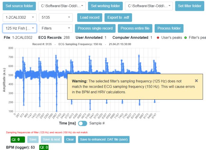
Figure 7.3: If there is a mis-match between the used ECG frequency used to record the data and the selected filter. The following message appears.
