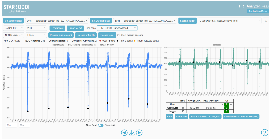
Figure 6.8: Processed ECG record graph in green (right) and original record in blue (left).
