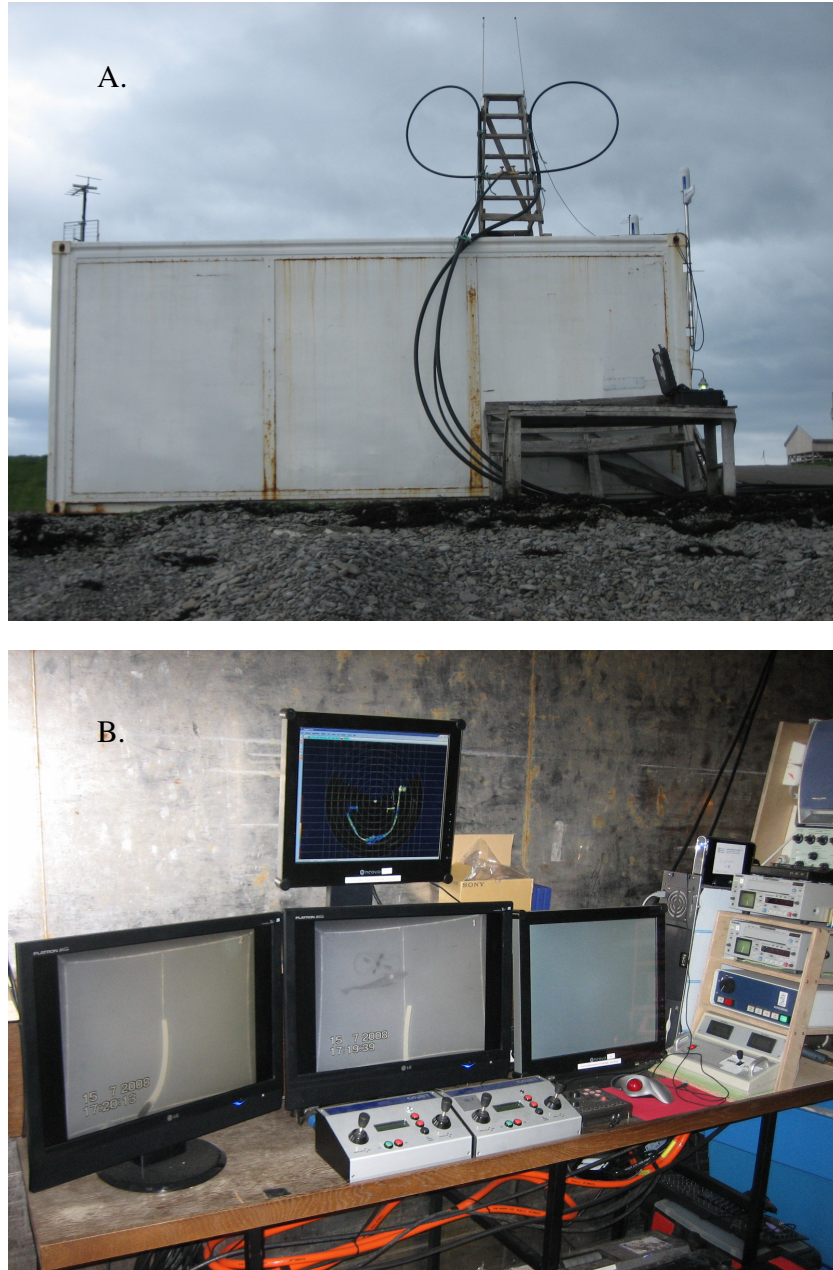
Figure 4. The control room. A. from outside showing the feeding system where seawater was pumped to two feeding pipes running from the roof of the container to the two feeding platforms (P1 and P2). The receivers for the video cameras can also be seen. B. from inside showing the screens of the video cameras monitoring the two feeding platforms (left), the sonar (above) and the videocamera attached to the sonar (right). A cod and a jellyfish can be seen on P1 and the feeding platforms and the netbag on the sonar. The equipment on the right was used to record the videos.
