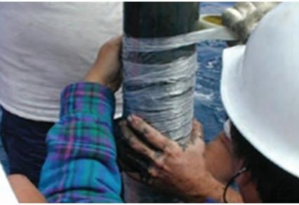
(H) Taping the core to keep its cylindrical (J) Labeling the core.
