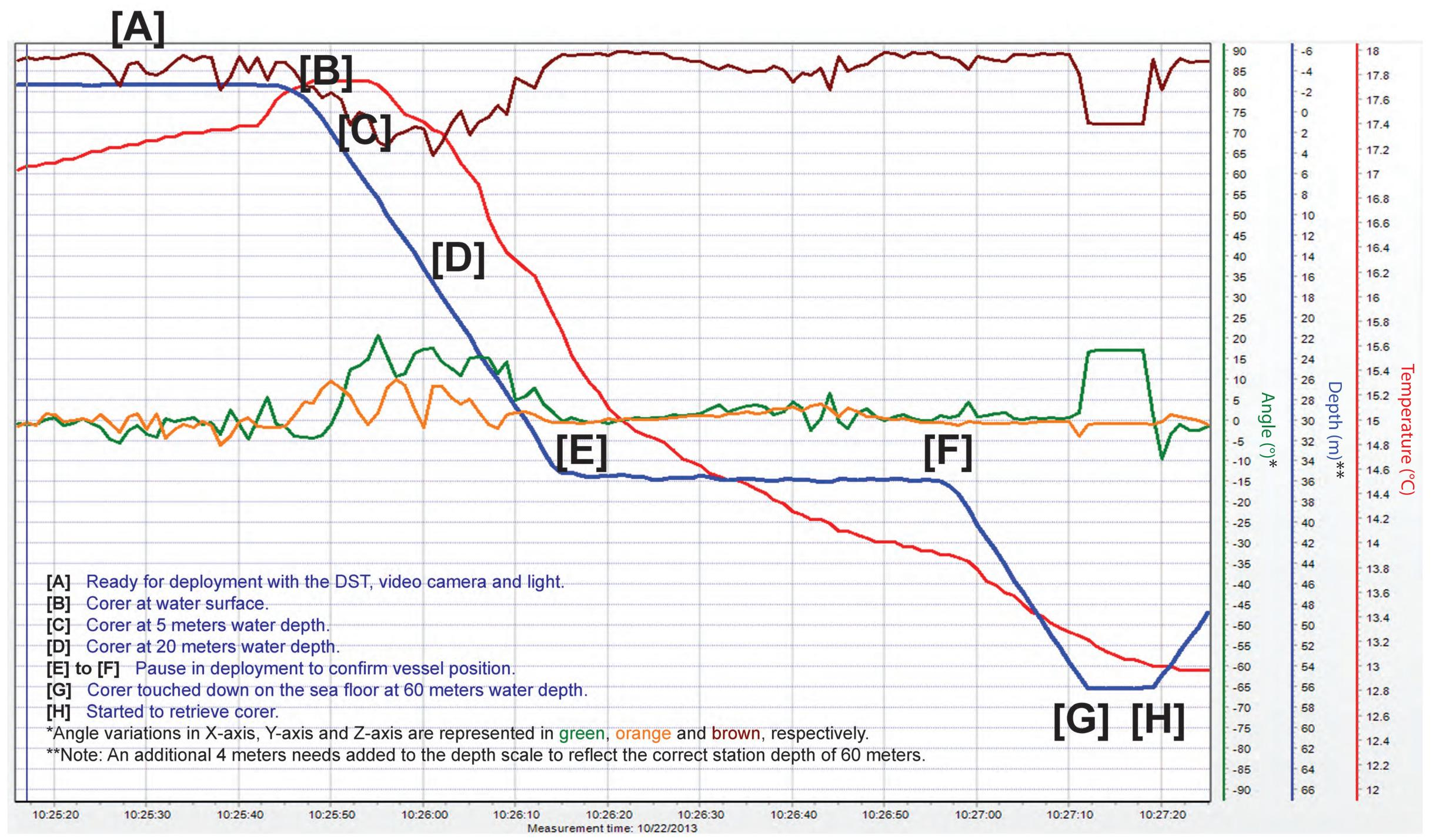
Based on video footage, the camera brace appeared to add drag to the coring device, causing an angled entry into the sediments (Figure 7). The tilt sensor confirmed the video interpretations: 38% of the cores needed resampling when the video camera brace was attached, compared to 8% of the cores that needed resampling without the brace.
