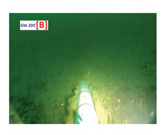
Figure 7 Deep Sediment Coring Conducted at Station 2DC on October 17, 2013. Core sampling event was rejected at station 2DC due to improper of angle penetration: the DST tag recorded 75 degree and 15 degree tilts on the X-axis and Z-axis respectively. These measurements were confirmed by the video footage of the slanted gravity corer (B).
