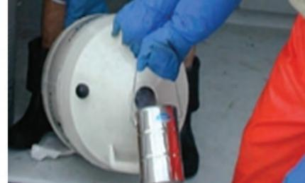
Fast freezing the core with liquid
