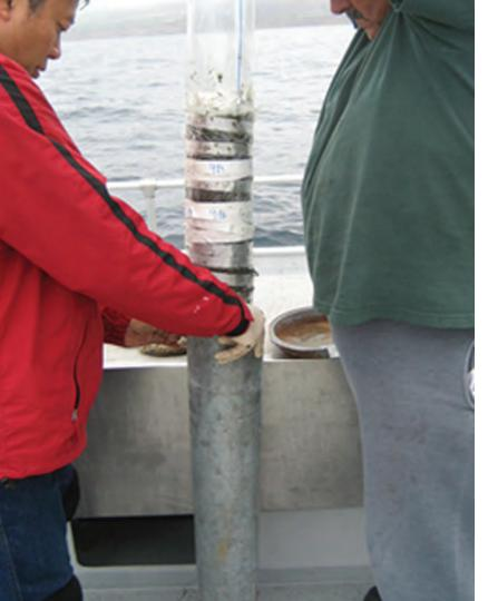
(K) Placing the core into a galvanized sleeve.
