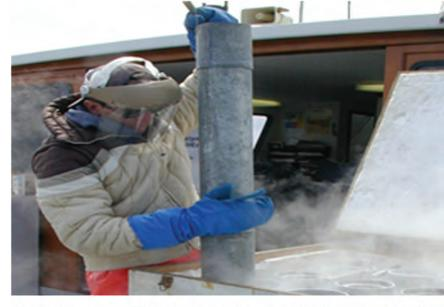
(M) Placing the core into a cold box with dry ice for preservation.
