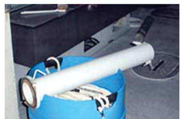
B) Empty barrel of the corer
