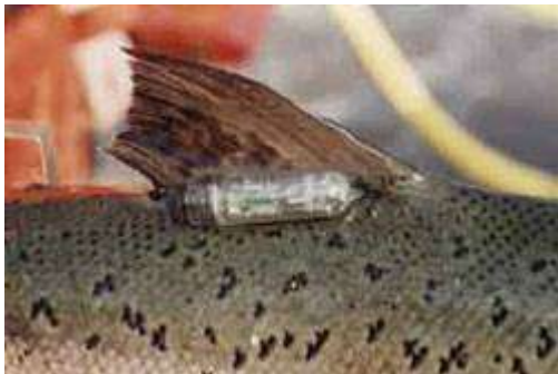
Fig. 1a. The data storage tag (DST 100) used in the study, externally attached to a salmon.
