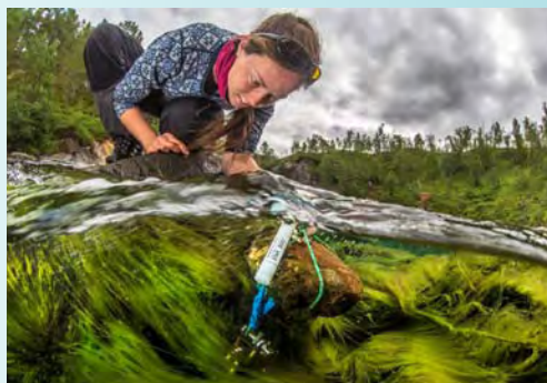
Starmon mini deployed in a river
