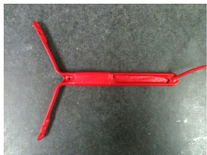
Fig. 1. Device to monitor vaginal temperature automatically in cattle. A blank CIDR is used to house the temperature logger, and the temperature logger is held in place by heat-activated shrink tubing. The entire device is then coated in multi-purpose rubber coating (Plasti Dip) to seal all components.
