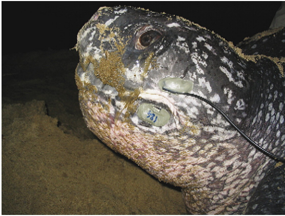
Fig. 1. Dermochelys coriacea . Photograph of a leatherback turtle head showing the positioning of the magnet (lower mandible) and hall sensor (upper mandible). The cable trailing from the sensor attaches to a data logging unit secured in the shoulder strap of a harness (photo: A Myers).
