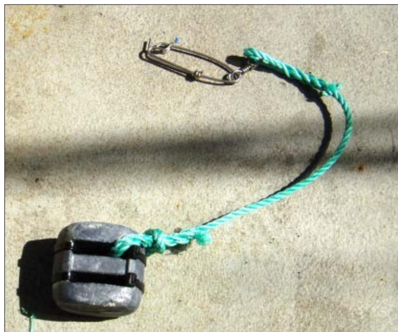
Figure 4: Three kilogram lead weight with swivel snap
