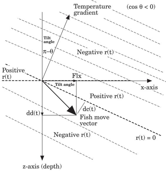
Figure 1. A fish move vector between two observations projected into a vertical plane through the temperature gradient  $\vec{\nabla T}$  (the  $xz$ -plane). The figure illustrates Equations (12) and (20).
