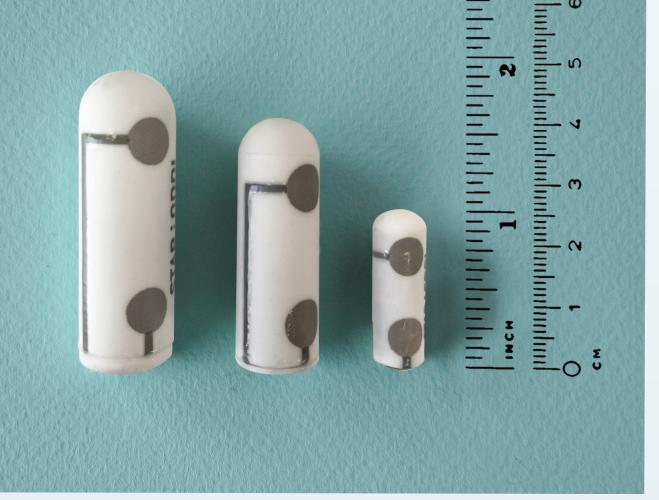
Centi-HRT 46x15mm and 19g Milli-HRT 13x39.5mm and 11.8g Micro-HRT 8.3x25.4mm and 3.3g\* \*Also available as a telemetry device
