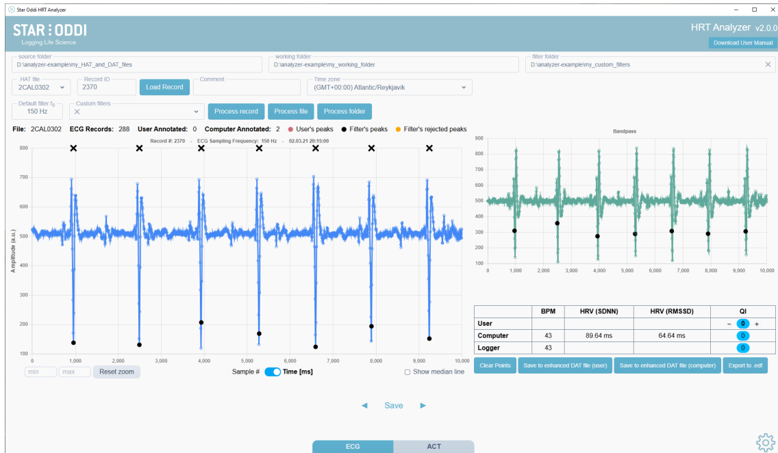
Figure 5.4: HRT Analyzer detected peaks are marked as black data points and X on top of the graph.
