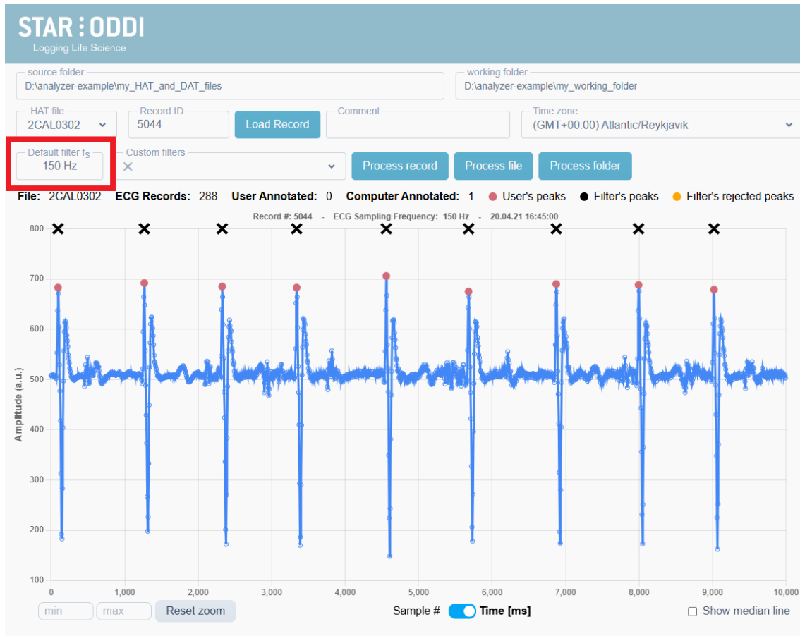
Figure 5.3: The sampling frequency of the built-in filter selected by the HRT Analyzer
