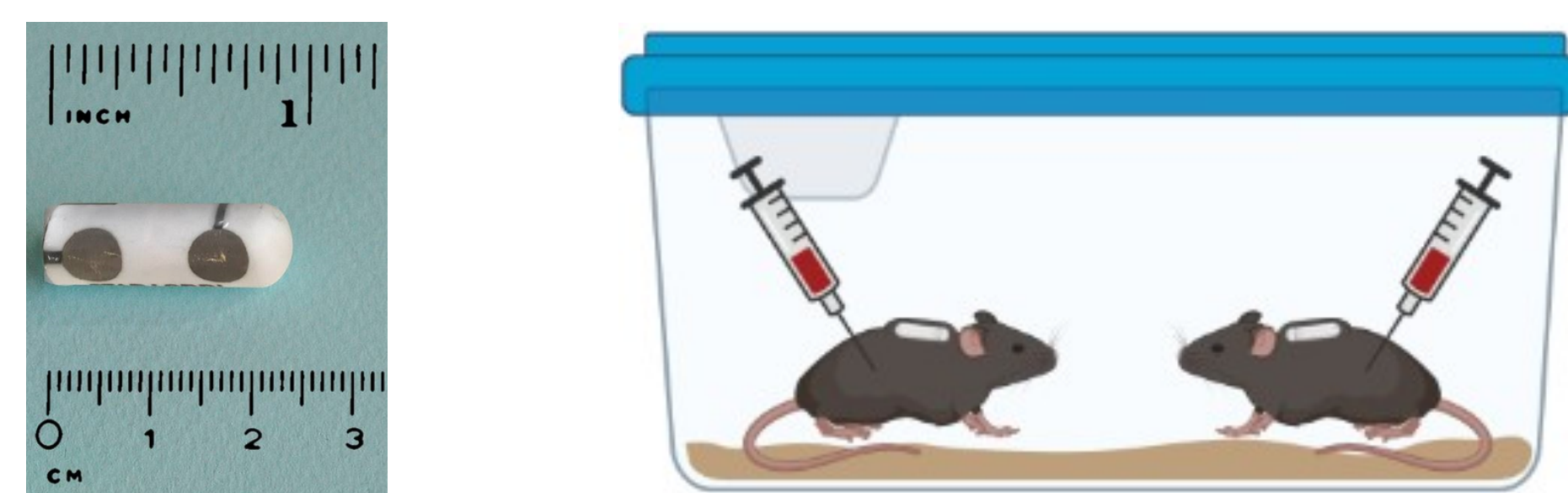
Figure 1: (Left) DST micro-HRT (3.3g), (right) example of location of logger, group housed animals that received an Isoproterenol injection in the end of study to elicit maximum heart rate.
